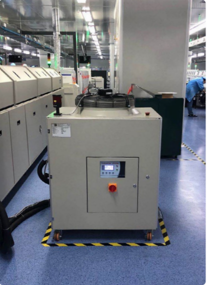
Nameplate power for a single unit: 5.5kw
